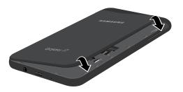
Press along the edge of the back cover until you have a secure seal.
