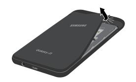
**Caution**: When removing the back cover, use the slot next to the Volume key to gently lift the cover off. Pulling on the Speaker (located next to the Power key) may cause damage.
